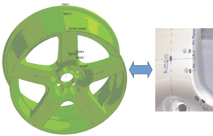
Strain measurement during wheel revolution
