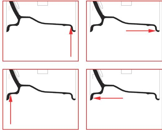
Derivation of strains from the Finite Element calculation at the strain gauge application areas
